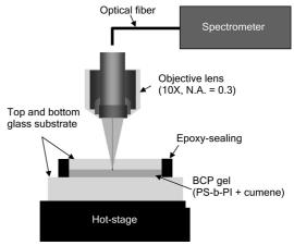
**Figure 1.** Schematic of the experimental setup for recording reflectivity vs wavelength as a function of sample temperature for the 1D PS-*b*-PI lamellar photonic gel.
