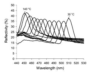
**Figure 2.** Measured normal incidence reflectivity spectra of the PSb-PI block copolymer lamellar photonic gel at 12 different temperatures between 30 and 140 °C in 10 °C increments.
